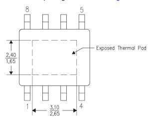
Figure 17. Thermal Pad Dimensions
