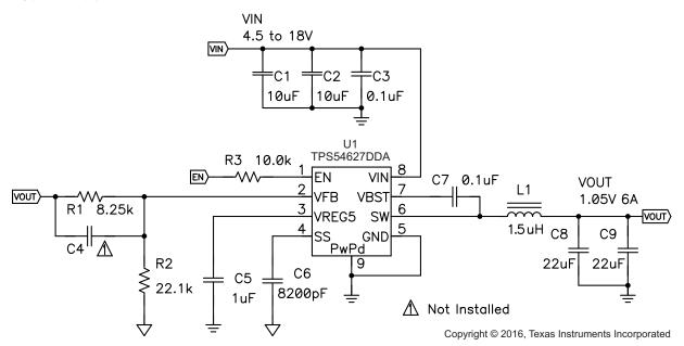
Figure 11. Simplified Application Schematic
