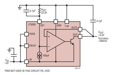
Figure 1. Basic Adjustable Regulator
