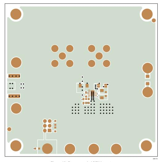
Figure 16. Recommended DFN Layout
