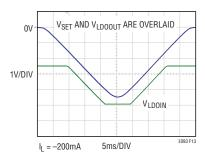
Figure 13. Ramping V<sub>SET</sub> from OV to -4.5V (and Back to OV)
