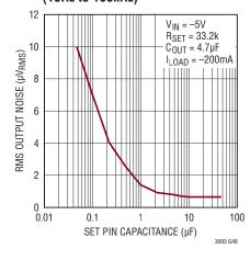
Integrated RMS Output Noise (10Hz to 100kHz)
