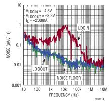
Figure 14. LT3093's Input and Output Noise Spectral Density
