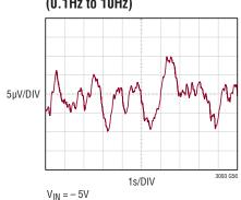
$V_{IN} = -5V$   $R_{SET} = 33.2k$   $C_{OUT} = 4.7\mu F$   $C_{SET} = 4.7\mu F$  $I_{LOAD} = -200 \text{mA}$
