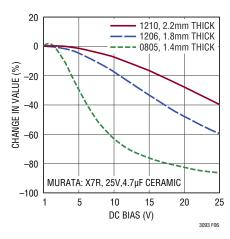
Figure 6. Capacitor Voltage Coefficient for Different Case Sizes
