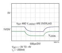
Figure 12. Stepping V<sub>SET</sub> from -3V to -4V (and Back to -3V)
