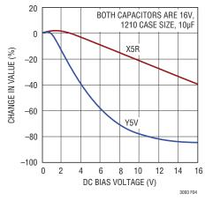
Figure 4. Ceramic Capacitor DC Bias Characteristics
