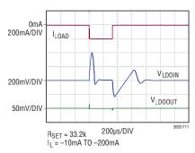
Figure 11. Load Step Response Using the VIOC Buffer
