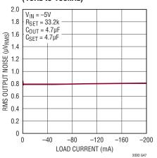
Integrated RMS Output Noise (10Hz to 100kHz)
