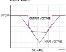
$$\begin{split} &V_{IN} = 0V \ T0 \ -5V \\ &V_{EN/UV} = V_{IN} \\ &R_{SET} = 33.2k \\ &C_{OUT} = 4.7 \mu F \\ &C_{SET} = 4.7 \mu F \\ &R_L = 16.5 \Omega \end{split}$$
