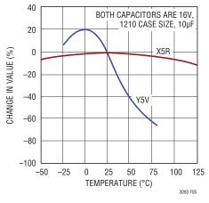
Figure 5. Ceramic Capacitor Temperature Characteristics
