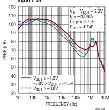
Power Supply Ripple Rejection
