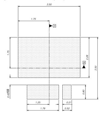
Figure 10. Recommended footprint (dimensions are in mm)
