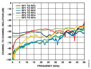
Figure 17. Channel to Channel Isolation vs. Frequency, RFC to RF2 Path On
