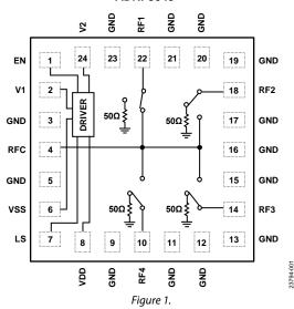
The ADRF5043 has enable and logic select controls to feature all off state and port mirroring, respectively.
