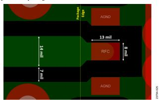
Figure 24. RF Trasmission Lines
