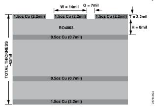
Figure 23. Evaluation Board Cross Sectional View
