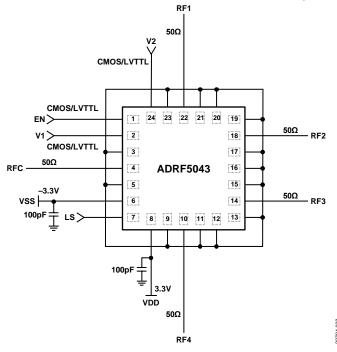
Figure 25. Application Circuit
