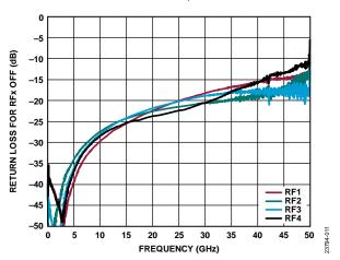
Figure 11. Return Loss for RFx Off vs. Frequency
