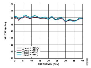
Figure 20. Input IP3 vs. Frequency over Various Temperatures
