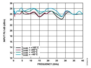
Figure 19. Input P0.1dB vs. Frequency over Various Temperatures
