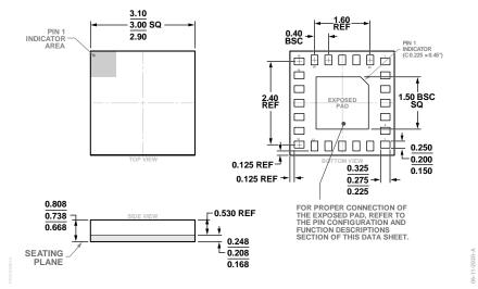
Figure 26. 24-Terminal Land Grid Array [LGA] 3 mm × 3 mm Body and 0.738 mm Package Height (CC-24-12) Dimensions shown in millimeters
