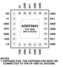
Figure 3. Pin Configuration (Top View)
