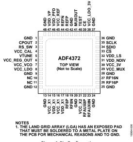
Figure 6. Pin Configuration
