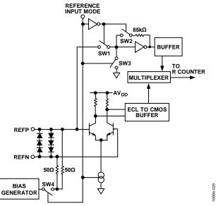
Figure 29. Reference Input Stage, Differential Mode
