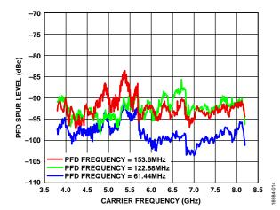
Figure 14. PFD Spurious Sweep,  $f_{PFD} = 61.44$  MHz, Loop Filter Bandwidth = 100 kHz
