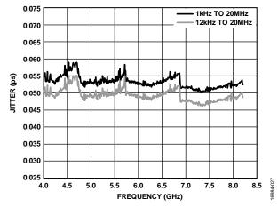
Figure 22. RMS Jitter, Fractional-N,  $f_{PFD} = 153.6 \text{ MHz}$ , VCC\_VCO = 5 V
