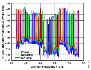
Figure 16. Integer Boundary Spurious Sweep vs. Carrier Frequency, f<sub>PFD</sub> = 61.44 MHz, 122.88 MHz, and 153.6 MHz, Loop Filter Bandwidth = 100 kHz
