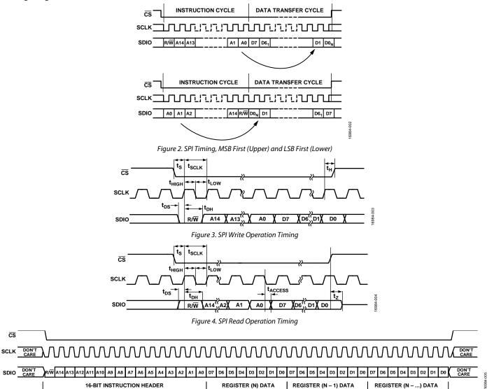
Figure 5. 3-Wire, MSB First, Descending Data, Streaming
