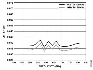
Figure 21. RMS Jitter, Integer-N, f<sub>PFD</sub> = 245.76 MHz, Loop Filter Bandwidth = 220 kHz, VCC\_VCO = 5 V
