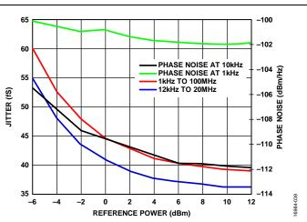
Figure 27. Jitter and Phase Noise,  $f_{PFD} = 250 \text{ MHz}$
