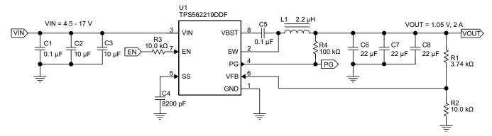
Figure 17. TPS562219 1.05V/2A Reference Design
