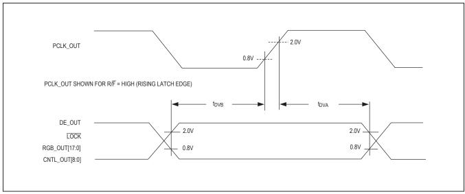
Figure 5. Synchronous Output Timing
