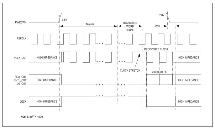
Figure 7. PLL Lock to REFCLK and Power-Down Delay
