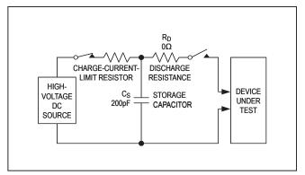
Figure 16. Machine Model ESD Test Circuit.
