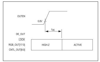
Figure 8. Output Enable Time
