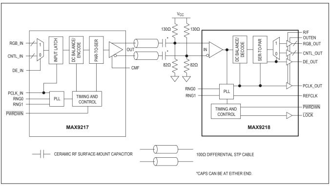
Figure 10. AC-Coupled Serializer and Deserializer with Two Capacitors per Link
