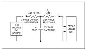
Figure 15. ISO 10605 Contact Discharge ESD Test Circuit
