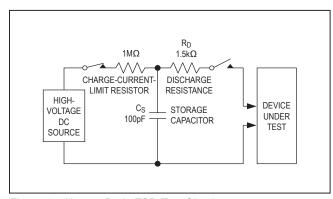
Figure 14. Human Body ESD Test Circuit
