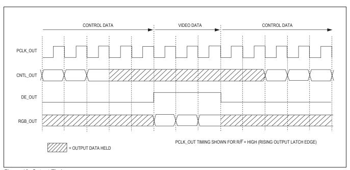
Figure 13. Output Timing
