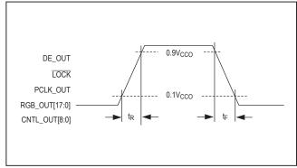
Figure 3. Output Rise and Fall Times
