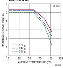
Derating, V<sub>OUT</sub> = 8V, BIAS = 5V, DC1868A Demo Board Both Channels at Same Load
