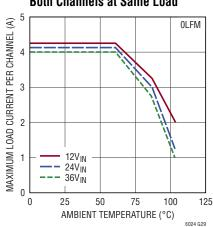
Derating, V<sub>OUT</sub> = 3.3V, BIAS = 5V, DC1868A Demo Board Channel 2 Off
