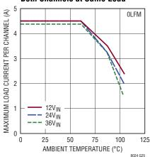
Derating, V<sub>OUT</sub> = 1.8V, BIAS = 5V, DC1868A Demo Board Channel 2 Off
