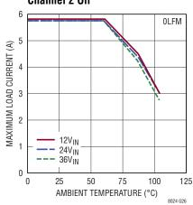
Derating, V<sub>OUT</sub> = 2.5V, BIAS = 5V, DC1868A Demo Board Both Channels at Same Load
