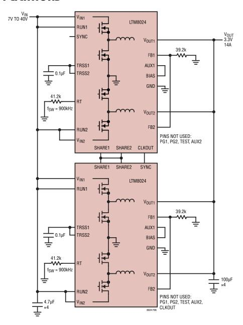
Figure 6. Parallel Four Channels to Produce 3.3V/14A from 7V to  $40 V_{\text{IN}}.$  BIAS is Tied to AUX1
