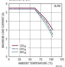
Derating, V<sub>OUT</sub> = 5V, BIAS = 5V, DC1868A Demo Board Both Channels at Same Load
