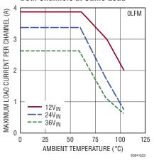
Derating, V<sub>OUT</sub> = 8V, BIAS = 5V, DC1868A Demo Board Channel 2 Off
