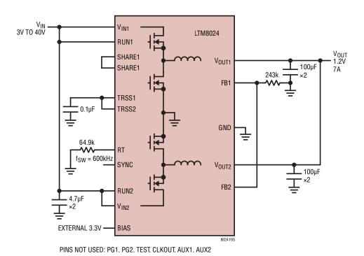
Figure 5. Parallel Two Channels to Produce 1.2V/7A from 3V to  $40V_{\text{IN}}$ . BIAS is Tied to External 3.3V
