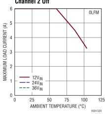
Derating, V<sub>OUT</sub> = 1.2V, BIAS = 5V, DC1868A Demo Board Both Channels at Same Load
