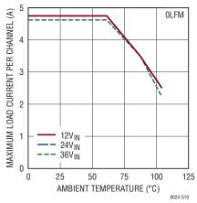
Derating, V<sub>OUT</sub> = 1V, BIAS = 5V, DC1868A Demo Board Channel 2 Off
