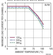
Derating, V<sub>OUT</sub> = 1.5V, BIAS = 5V, DC1868A Demo Board Channel 2 Off
