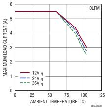
Derating, V<sub>OUT</sub> = 3.3V, BIAS = 5V, DC1868A Demo Board Both Channels at Same Load
