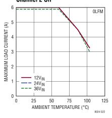
Derating, V<sub>OUT</sub> = 1.5V, BIAS = 5V, DC1868A Demo Board Both Channels at Same Load
