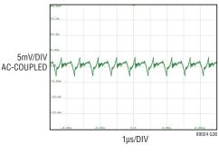
$V_{IN} = 12V$ ,  $V_{OUT} = 3.3V$  $I_{OUT} = 3.5A$ ,  $f_{SW} = 900kHz$
