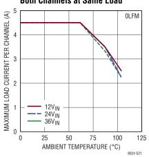
Derating, V<sub>OUT</sub> = 1.2V, BIAS = 5V, DC1868A Demo Board Channel 2 Off
