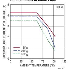
Derating, V<sub>OUT</sub> = 5V, BIAS = 5V, DC1868A Demo Board Channel 2 Off
