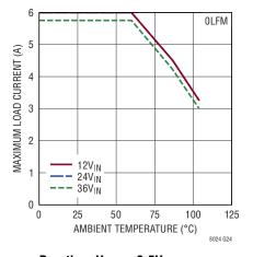
Derating, V<sub>OUT</sub> = 1.8V, BIAS = 5V, DC1868A Demo Board Both Channels at Same Load
