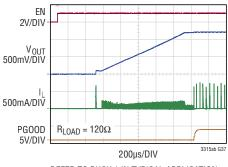
REFER TO BUCK 1 IN TYPICAL APPLICATION: DUAL 1.2V AND 0.8V 2MHz, 2A BUCK REGULATORS,  $V_{IN}$  = 3.3V
