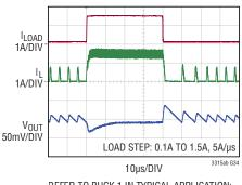
REFER TO BUCK 1 IN TYPICAL APPLICATION: DUAL 1.2V AND 0.8V 2MHz, 2A BUCK REGULATORS,  $V_{\rm IN}$  = 3.3V
