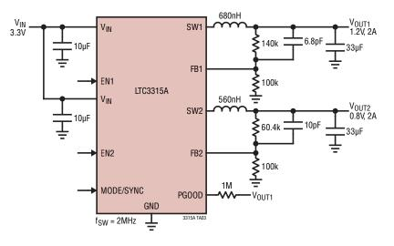
Dual 1.2V and 0.8V 2MHz, 2A Buck Regulators,  $V_{\text{IN}}$  = 3.3V
