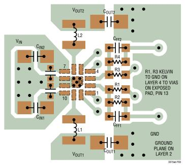
Figure 3. Recommended LTC3315A LQFN PCB Layout
