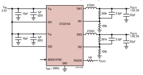
Dual 1.5V and 1.8V 2MHz, 2A Buck Regulators,  $V_{\text{IN}}$  = 2.5V
