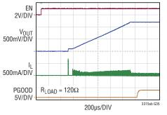
REFER TO BUCK 1 IN TYPICAL APPLICATION: DUAL 1.2V AND 0.8V 2MHz, 2A BUCK REGULATORS,  $V_{IN}$  = 3.3V
