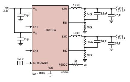
Dual 1.2V and 0.8V 1MHz, 2A Buck Regulators,  $V_{\text{IN}}$  = 3.3V
