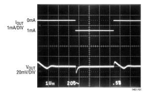
Figure 1. 1mA Load Step with  $C_L = 1\mu F$
