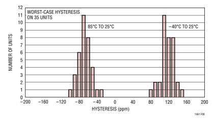
Figure 8. -40°C to 85°C Hysteresis of 35 Parts Soldered Onto a PC Board
