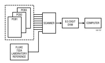
Figure 7. Long-Term Drift Measurement Setup
