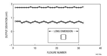
Figure 5a. Two Typical LT1461S8-2.5s, Vertical Orientation without Slots
