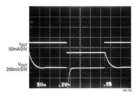
Figure 2. 50mA Load Step with  $C_L = 2\mu F$
