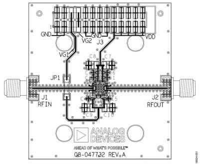
Figure 52. EV1HMC1114PM5 (08-047732) Evaluation Board PCB
