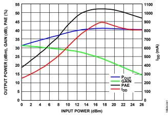
Figure 41. Output Power, Gain, PAE, and IDD vs. Input Power at 3.8 GHz
