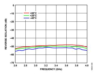
Figure 36. Reverse Isolation vs. Frequency at Various Temperatures
