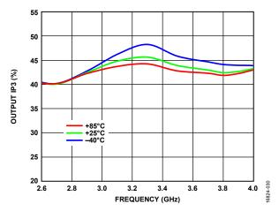
Figure 30. Output IP3 vs. Frequency at Various Temperatures,  $P_{\text{OUT}}$  per Tone = 30 dBm
