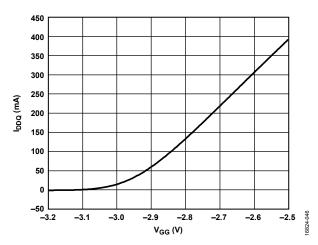
Figure 46.  $I_{DDQ}$  vs.  $V_{GG}$  at  $V_{DD} = 28$  V, Representative of a Typical Device
