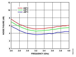
Figure 44. Noise Figure vs. Frequency at Various Temperatures
