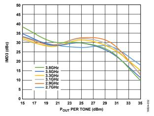
Figure 32. Output Third-Order Intermodulation (IMD3) vs.  $P_{OUT}$  per Tone,  $V_{DD} = 24 \text{ V}$
