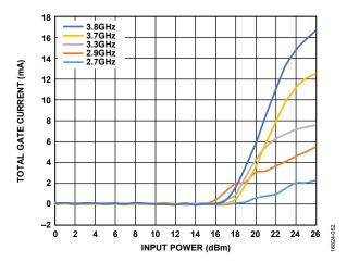
Figure 49. Total Gate Current vs. Input Power at Various Frequencies,  $V_{DD}$  = 28 V
