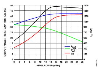
Figure 37. Output Power, Gain, PAE, and  $I_{DD}$  vs. Input Power at 2.9 GHz
