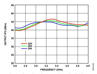
Figure 28. Output IP3 vs. Frequency at Various Supply Voltages,  $P_{OUT}$  per Tone = 30 dBm
