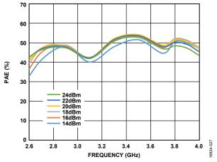
Figure 27. PAE vs. Frequency at Various Input Powers
