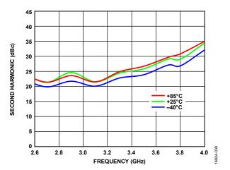
Figure 39. Second Harmonic vs. Frequency at Various Temperatures,  $P_{OUT} = 30 \text{ dBm}$
