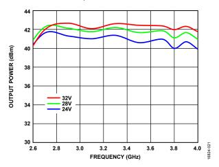
Figure 21. Output Power vs. Frequency at Various Supply Voltages, Input Power = 18 dBm
