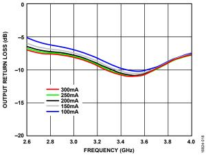
Figure 18. Output Return Loss vs. Frequency at Various Quiescent Currents
