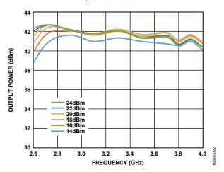
Figure 22. Output Power vs. Frequency at Various Input Powers
