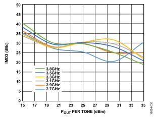
Figure 35. IMD3 vs.  $P_{OUT}$  per Tone,  $V_{DD} = 28 \text{ V}$
