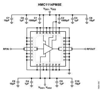
Figure 51. Typical Application Circuit
