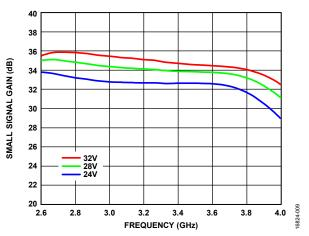
Figure 9. Small Signal Gain vs. Frequency at Various Supply Voltages
