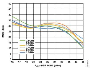
Figure 33. IMD3 vs.  $P_{OUT}$  per Tone,  $V_{DD} = 32 V$
