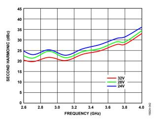
Figure 42. Second Harmonic vs. Frequency at Various Supply Voltages,  $P_{OUT} = 30 \text{ dBm}$
