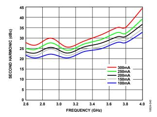
Figure 40. Second Harmonic vs. Frequency at Various Quiescent Currents,  $P_{OUT} = 30 \text{ dBm}$
