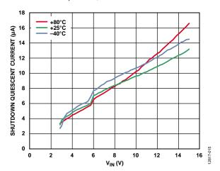
Figure 14. Shutdown Quiescent Current (I<sub>SHDN</sub>) vs. Input Voltage (V<sub>IN</sub>) for Various Temperatures, EN Pin Below Shutdown Threshold
