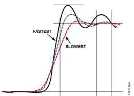
Figure 22. Switching Node at Various Slew Rate Settings
