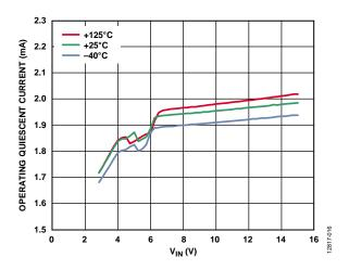
Figure 15. Operating Quiescent Current (I<sub>O</sub>) vs. Input Voltage (V<sub>IN</sub>) for Various Temperatures, EN Pin On
