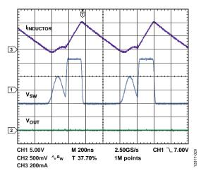
Figure 19. Discontinuous Conduction Mode Operation Showing Inductor Current ( $I_{INDUCTOR}$ ), Switch Node Voltage ( $V_{SW}$ ), and Output Ripple ( $V_{OUT}$ ),  $V_{IN} = 12 V$ ,  $V_{OUT} = -5 V$ ,  $I_{LOAD} = 50 \text{ mA}$ ,  $f_{SW} = 1.2 \text{ MHz}$ ,  $T_A = 25^{\circ}\text{C}$
