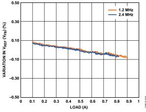
Figure 11. Load Regulation,  $V_{IN} = 12 \text{ V}$ ,  $V_{OUT} = -5 \text{ V}$ ,  $f_{SW} = 1.2 \text{ MHz}$ ,  $T_A = 25 ^{\circ}\text{C}$  (Skip Mode Not Shown)
