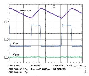
Figure 20. Continuous Conduction Mode Operation Showing Inductor Current ( $I_{INDUCTOR}$ ), Switch Node Voltage ( $V_{SW}$ ), and Output Ripple ( $V_{OUT}$ ),  $V_{IN} = 12 \text{ V}$ ,  $V_{OUT} = -5 \text{ V}$ ,  $I_{LOAD} = 200 \text{ mA}$ ,  $f_{SW} = 1.2 \text{ MHz}$ ,  $T_A = 25 ^{\circ}\text{C}$
