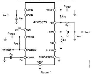
Other key safety features in the ADP5073 include overcurrent protection (OCP), overvoltage protection (OVP), thermal shutdown (TSD), and input undervoltage lockout (UVLO).
