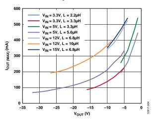
Figure 4. Maximum Output Current,  $f_{SW} = 2.4$  MHz,  $T_A = 25$ °C, Based on Target of 70%  $I_{LIM \, (MIN)}$
