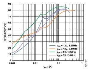
Figure 7. Efficiency vs. Current Load ( $I_{OUT}$ ),  $V_{IN} = 12 \text{ V}$  and 5 V,  $V_{OUT} = -15 \text{ V}$ ,  $T_A = 25^{\circ}\text{C}$
