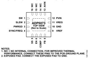
Figure 2. Pin Configuration
