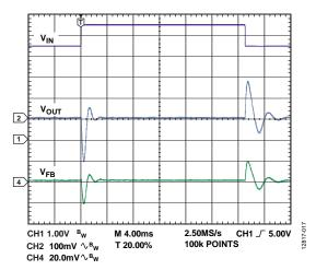
Figure 16. Line Transient Showing  $V_{IN}$ ,  $V_{OUT}$ , and  $V_{FB}$ ,  $V_{IN}=4.5$  V to 5.5 V Step,  $V_{OUT}=-5$  V,  $R_{LOAD}=300$   $\Omega$ ,  $f_{SW}=1.2$  MHz,  $T_A=25$ °C
