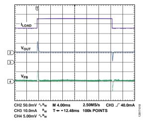
Figure 17. Load Transient Showing  $I_{LOAD}$ ,  $V_{OUT}$ , and  $V_{FB}$ ,  $V_{IN} = 12$  V,  $V_{OUT} = -5$  V,  $I_{LOAD} = 35$  mA to 45 mA Step,  $f_{SW} = 1.2$  MHz,  $T_A = 25$  °C
