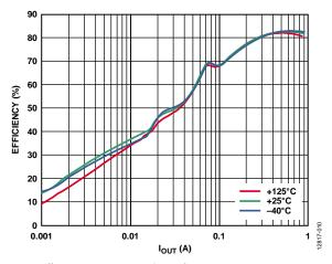
Figure 9. Efficiency vs. Current Load ( $I_{OUT}$ ) for Various Temperatures,  $V_{IN} = 5 V$ ,  $V_{OUT} = -15 V$ ,  $f_{SW} = 1.2 \text{ MHz}$
