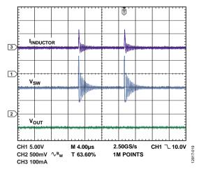
Figure 18. Skip Mode Operation Showing Inductor Current ( $I_{INDUCTOR}$ ), Switch Node Voltage ( $V_{SW}$ ), and Output Ripple ( $V_{OUT}$ ),  $V_{IN} = 12 V$ ,  $V_{OUT} = -5 V$ ,  $I_{LOAD} = 1 \text{ mA}$ ,  $f_{SW} = 1.2 \text{ MHz}$ ,  $T_A = 25 ^{\circ}\text{C}$
