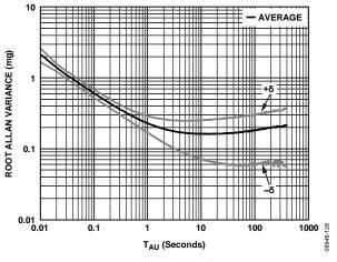
Figure 8. Accelerometer Root Allan Variance
