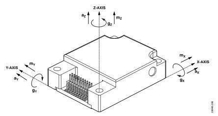
Figure 18. Inertial Sensor Direction Reference
