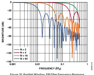
Figure 20. Bartlett Window, FIR Filter Frequency Response (Phase Delay = N Samples)
