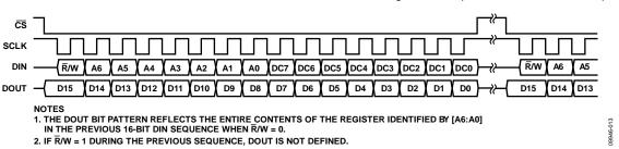
Figure 12. SPI Communication Bit Sequence
