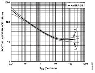
Figure 7. Gyroscope Root Allan Variance
