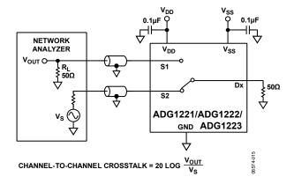
Figure 30. Test Circuit 8—Channel-to-Channel Crosstalk
