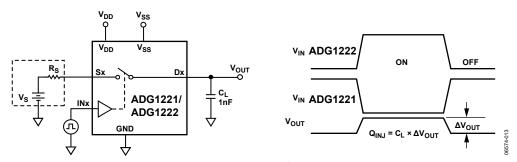
Figure 28. Test Circuit 6—Charge Injection
