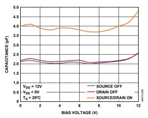
Figure 21. Capacitance vs. Bias Voltage
