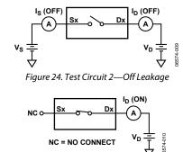
Figure 25. Test Circuit 3—On Leakage
