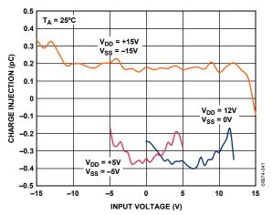
Figure 2. Charge Injection vs. Input Voltage
