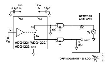
Figure 29. Test Circuit 7—Off Isolation
