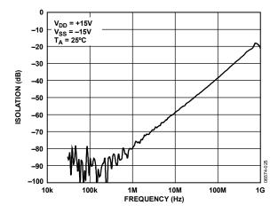
Figure 15. Off Isolation vs. Frequency
