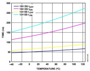
Figure 14. t<sub>ON</sub>/t<sub>OFF</sub> vs. Temperature
