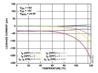
Figure 10. Leakage Current as a Function of Temperature, Dual Supply
