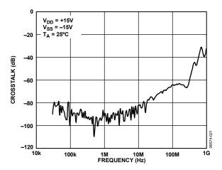
Figure 16. Crosstalk vs. Frequency
