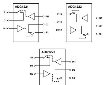
SWITCHES SHOWN FOR A LOGIC 0 INPUT Figure 1.
