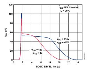
Figure 12. IDD vs. Logic Level
