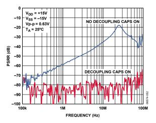
Figure 18. ACPSRR vs. Frequency
