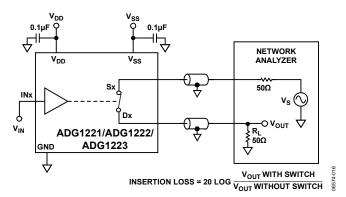
Figure 31. Test Circuit 9—Bandwidth
