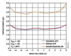
Figure 22. Capacitance vs. Bias Voltage
