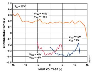
Figure 13. Charge Injection vs. Input Voltage
