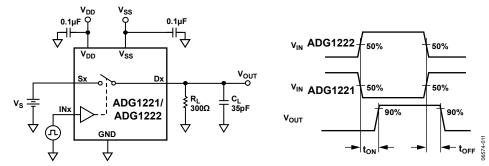
Figure 26. Test Circuit 4—Switching Times
