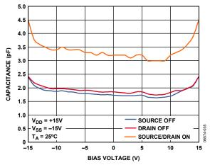
Figure 20. Capacitance vs. Bias Voltage
