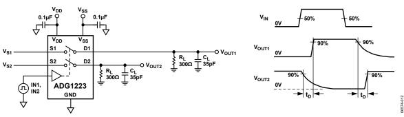
Figure 27. Test Circuit 5—Break-Before-Make Time Delay
