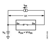
Figure 23. Test Circuit 1—On Resistance
