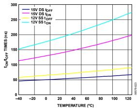
Figure 13. ton/toff Times vs. Temperature
