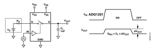
Figure 27. Charge Injection
