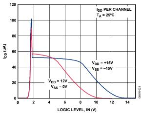
Figure 11. IDD vs. Logic Level, IN
