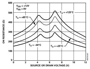
Figure 7. On Resistance vs. Source or Drain Voltage, Different Temperatures, Single Supply
