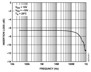
Figure 15. Insertion Loss vs. Frequency
