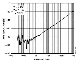
Figure 14. Off Isolation vs. Frequency
