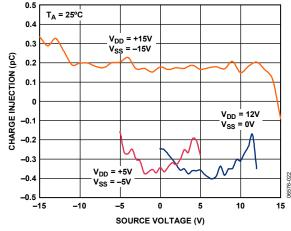
Figure 12. Charge Injection vs. Source Voltage
