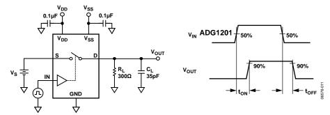
Figure 26. Switching Times
