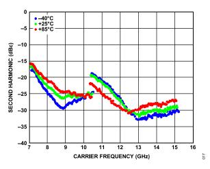
Figure 12. Second Harmonic vs. Carrier Frequency at RFOUT, Maximum
