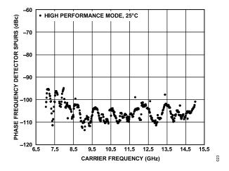
Figure 16. Phase Frequency Detector Spurs vs. Carrier Frequency, 100
