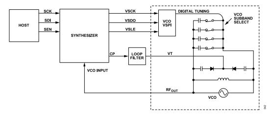
Figure 20. Simplified Step Tuned VCO
