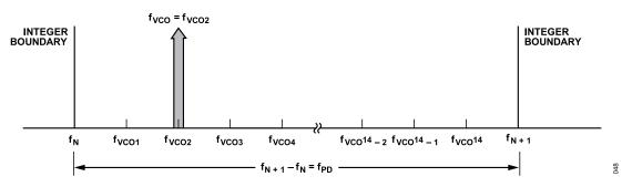
Figure 26. Exact Frequency Tuning
