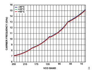
Figure 8. Carrier Frequency vs. VCO Band, Autocalibration Enabled, VDDLS = 3.3 V, VPPCP = 3.3 V
