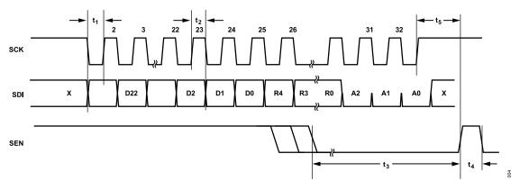
Figure 30. Open Mode: Serial Port Timing Diagram, Write Cycle
