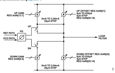
Figure 24. Charge Pump Gain and Offset Control
