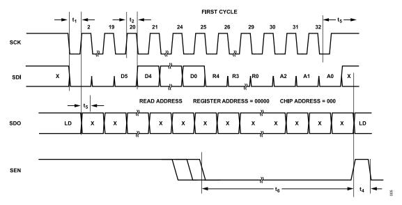
Figure 31. Open Mode: Serial Port Timing Diagram, Read Operation, First Cycle
