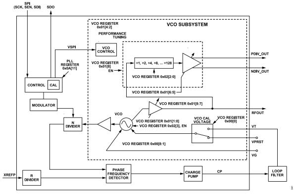
Figure 19. Detail of PLL and VCO Subsystems
