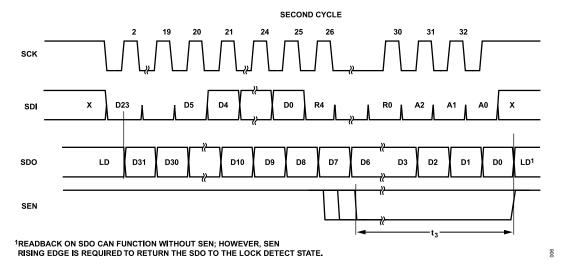
Figure 32. Open Mode: Serial Port Timing Diagram, Read Operation, Second Cycle
