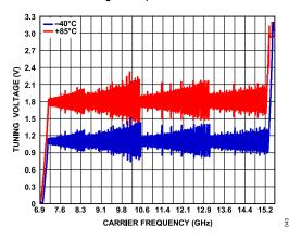
Figure 21. Tuning Voltage vs. Carrier Frequency After Calibration, Maximum Tuning Resolution, Register 0x0A, Bits[2:0] = 7
