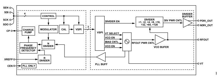
Figure 18. PLL and VCO Subsystems
