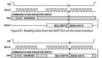
Figure 82. Writing Data to the ADE7763 via the Serial Interface
