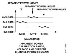
Figure 65. Apparent Power Calculation Output Range
