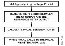
Figure 75. Calibrating Phase Using a Reference Meter
