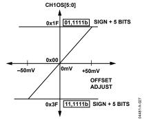
Figure 26. Channel 1 Offset Correction Range (Gain = 1)
