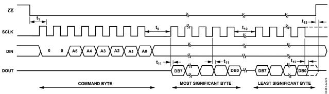
Figure 85. Serial Interface Read Timing
