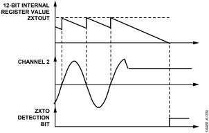
Figure 33. Zero-Crossing Timeout Detection
