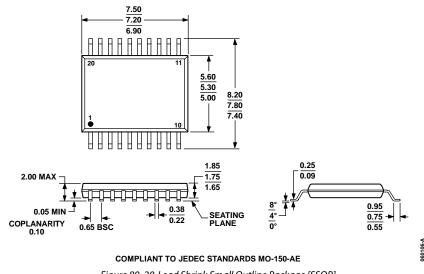
Figure 89. 20-Lead Shrink Small Outline Package [SSOP] (RS-20) Dimensions shown in millimeters
