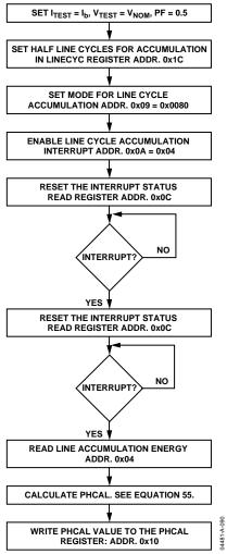
Figure 76. Calibrating Phase with an Accurate Source
