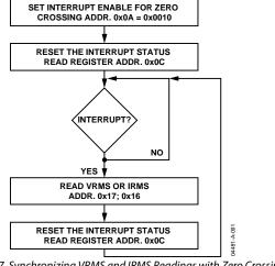
Figure 77. Synchronizing VRMS and IRMS Readings with Zero Crossings
