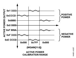
Figure 56. Active Power Calculation Output Range
