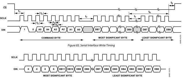
Figure 84. 12-Bit Serial Write Operation
