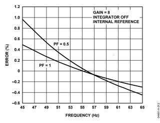
Figure 12. Active Energy Error as a Percentage of Reading (Gain = 8) over Frequency with Internal Reference and Integrator Off
