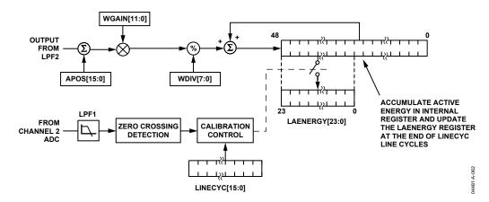
Figure 61. Energy Calculation Line Cycle Energy Accumulation Mode
