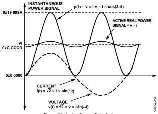
Figure 53. Active Power Calculation
