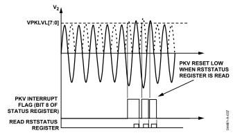
Figure 36. Peak Level Detection
