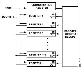
Figure 80. Addressing ADE7763 Registers via the Communication Register
