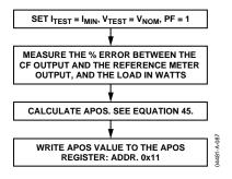
Figure 73. Calibrating Watt Offset Using a Reference Meter
