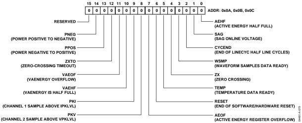
Figure 87. Interrupt Status/Interrupt Enable Register
