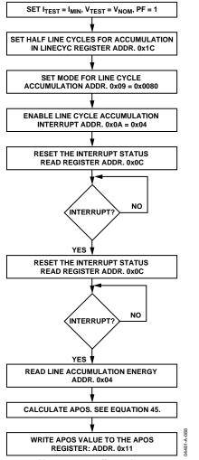
Figure 74. Calibrating Watt Offset with an Accurate Source
