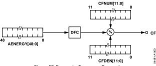
Figure 59. Energy-to-Frequency Conversion
