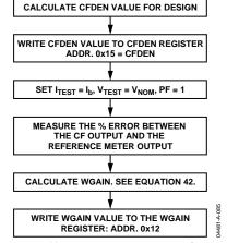
Figure 71. Calibrating Watt Gain Using a Reference Meter
