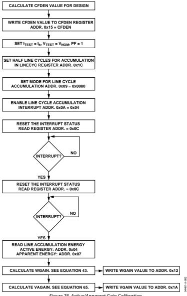
Figure 78. Active/Apparent Gain Calibration
