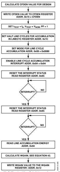
Figure 72. Calibrating Watt Gain Using an Accurate Source
