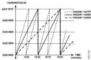
Figure 67. Energy Register Rollover Time for Full-Scale Power (Maximum and Minimum Power Gain)
