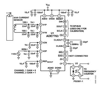
Figure 21. Test Circuit for Performance Curves with Integrator On
