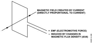
Figure 27. Principle of a di/dt Current Sensor
