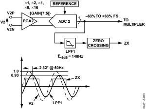
Figure 32. Zero-Crossing Detection on Channel 2
