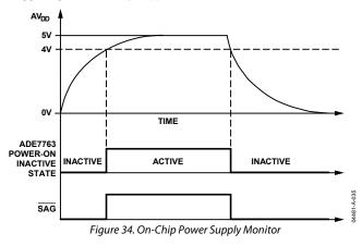
As seen in Figure 34, the trigger level is nominally set at 4 V. The tolerance on this trigger level is about  $\pm 5\%$ . The  $\overline{SAG}$  pin can also be used as a power supply monitor input to the MCU. The  $\overline{SAG}$  pin goes logic low when the ADE7763 is in its inactive state. The power supply and decoupling for the part should be such that the ripple at AVDD does not exceed 5 V  $\pm$  5%, as specified for normal operation.
