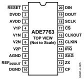
Figure 5. Pin Configuration (SSOP Package)
