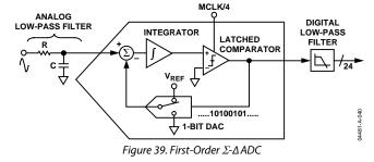
A  $\Sigma$ - $\Delta$  modulator converts the input signal into a continuous serial stream of 1s and 0s at a rate determined by the sampling clock. In the ADE7763, the sampling clock is equal to CLKIN/4. The 1-bit DAC in the feedback loop is driven by the serial data stream. The DAC output is subtracted from the input signal. If the loop gain is high enough, the average value of the DAC
