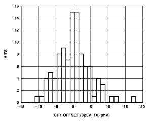
Figure 20. Channel 1 Offset (Gain = 1)
