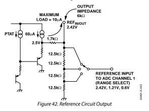
The REF<sub>IN/OUT</sub> pin can be overdriven by an external source such as a 2.5 V reference. Note that the nominal reference value supplied to the ADCs is now 2.5 V, not 2.42 V, which increases the nominal analog input signal range by  $2.5/2.42 \times 100\% = 3\%$  or from 0.5 V to 0.5165 V.
