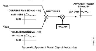
The gain of the apparent energy can be adjusted by using the multiplier and VAGAIN register (VAGAIN[11:0]). The gain is adjusted by writing a twos complement, 12-bit word to the VAGAIN register. Equation 25 shows how the gain adjustment is related to the contents of the VAGAIN register.
