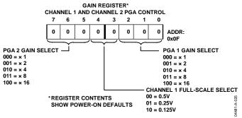
Figure 24. Analog Gain Register
