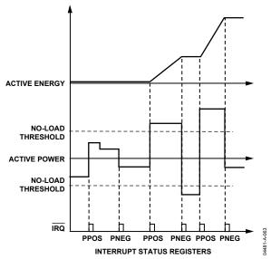
Figure 62. Energy Accumulation in Positive-Only Accumulation Mode
