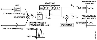
Figure 57. Active Power Signal Processing
