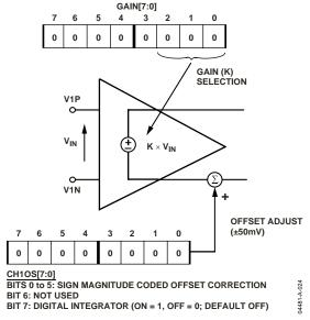
Figure 23. PGA in Channel 1
