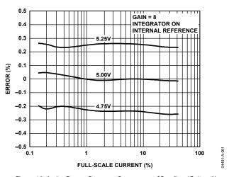
Figure 18. Active Energy Error as a Percentage of Reading (Gain = 8) over Power Supply with Internal Reference and Integrator On
