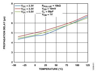
Figure 11. Propagation Delay vs. Temperature, Low to High,  $V_{\text{OD}} = 10 \text{ mV}$
