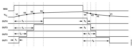
Figure 28. Mirrored Voltage Sequencer Timing Diagram
