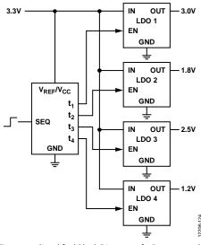
Figure 25. Simplified Block Diagram of a Programmable Sequencing Control Circuit
