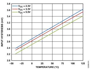
Figure 10. Input Hysteresis vs. Temperature for Various Supply Voltages  $(V_{CC})$ ,  $V_{CM} = 1 \text{ V}$
