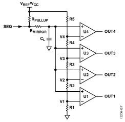
Figure 27. Circuit Configuration for a Mirrored Voltage Sequencer
