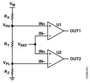
Figure 22. Positive Undervoltage/Overvoltage Monitoring Configuration
