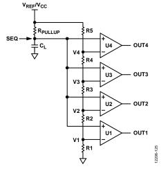
Figure 24. Programmable Sequencing Control Circuit
