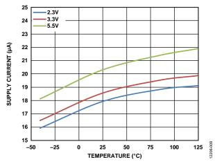
Figure 12. Supply Current vs. Temperature at Output Low Voltage for Various Supply Voltages (Vcc)
