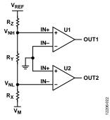
Figure 23. Negative Undervoltage/Overvoltage Monitoring Configuration
