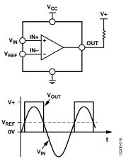
Figure 19. Basic Comparator and Input and Output Signals
