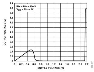
Figure 7. Output Voltage ( $V_{OUT}$ ) vs. Supply Voltage ( $V_{CC}$ ),  $R_{PULLUP} = 10 \text{ k}\Omega$
