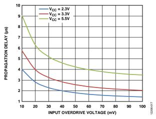
Figure 17. Propagation Delay vs. Input Overdrive Voltage, High to Low
