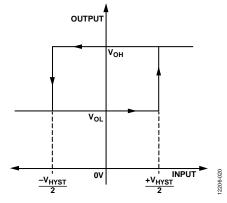
Figure 20. Comparator Hysteresis Transfer Function
