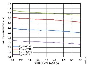
Figure 13. Input Hysteresis vs. Supply Voltage (Vcc) for Various Temperatures, Vcm = 1 V
