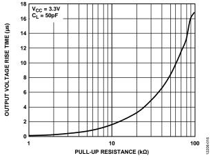
Figure 16. Output Voltage Rise Time (t<sub>R</sub>) vs. Pull-Up Resistance (R<sub>PULLUP</sub>)
