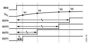
Figure 26. Programmable Sequencing Control Circuit Timing Diagram
