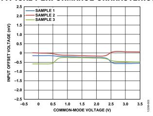
Figure 3. Input Offset Voltage ( $V_{CS}$ ) vs. Common-Mode Voltage ( $V_{CM}$ ),  $V_{CC} = 3.3 \text{ V}$
