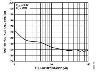
Figure 18. Output Voltage Fall Time (t<sub>F</sub>) vs. Pull-Up Resistance (R<sub>PULLUP</sub>)
