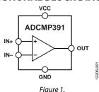
The ADCMP391 features a common-mode input voltage range of 200 mV beyond rails, an offset voltage of 1 mV typical across the full common-mode range, and a UVLO monitor. In addition, the design of the comparator allows a defined output state upon power-up. The comparator generates a logic low output if the supply voltage is less than the UVLO threshold.
