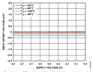
Figure 6. Input Offset Voltage ( $V_{CS}$ ) vs. Supply Voltage ( $V_{CC}$ ),  $V_{CM} = 1 V$  for Various Temperatures
