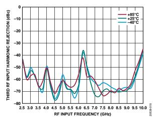
Figure 15. Third RF Input Harmonic Rejection vs. RF Input Frequency and Temperature
