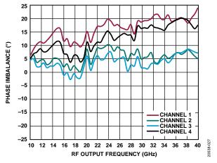
Figure 26. Phase Imbalance vs. RF Output Frequency
