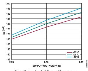
Figure 10. Icc vs. Supply Voltage and Temperature
