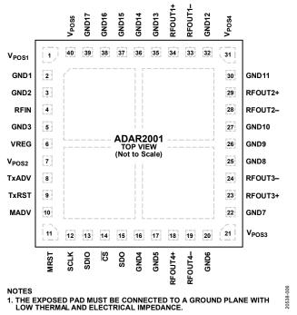
Figure 6. Pin Configuration (Top View, Not to Scale)
