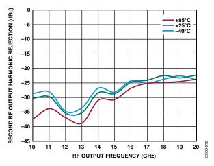
Figure 16. Second RF Output Harmonic Rejection vs. RF Output Frequency and Temperature
