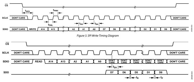
Figure 4. SPI 4-Wire Read Timing Diagram
