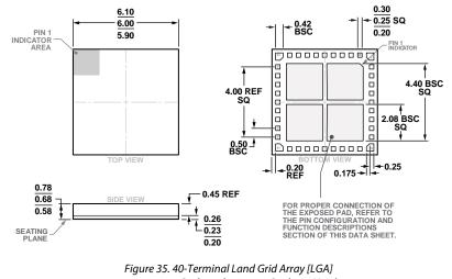
Figure 35. 40-1 erminal Land Grid Array [LGA] 6 mm × 6 mm Body and 0.75 mm Package Height (CC-40-7) Dimensions shown in millimeters
