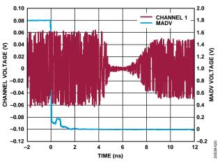
Figure 18. 25 GHz RF Frequency Band Switching with MADV
