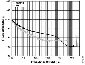
Figure 8. Phase Noise (OUT2)— $f_{OUT2} = 156.25 \text{ MHz}$  (HSTL)
