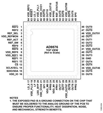
Figure 4. Pin Configuration
