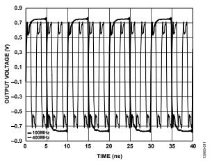
Figure 11. OUT8 Output Waveform, HCSL (100 MHz, 400 MHz)
