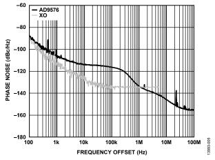
Figure 5. Phase Noise (OUT0)— $f_{OUT0} = 644.53125$  MHz (HSTL), Fractional
