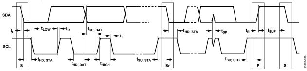
Figure 38. I<sup>2</sup>C Serial Port Timing
