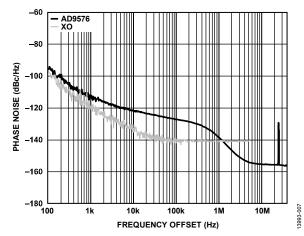
Figure 7. Phase Noise (OUT4)— $f_{OUT4} = 312.5 \text{ MHz}$  (LVDS)
