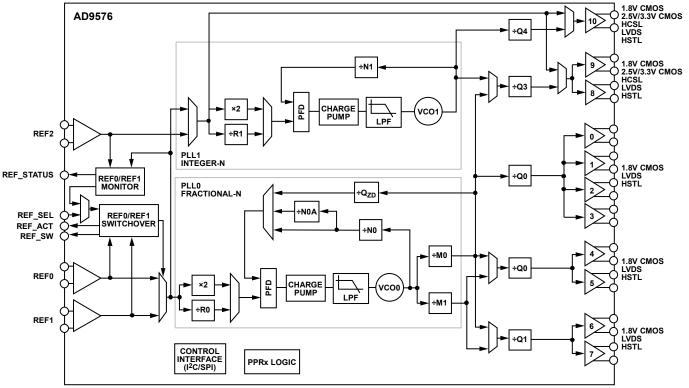
Figure 20. Detailed Functional Block Diagram
