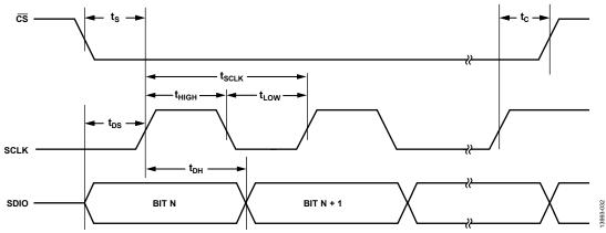
Figure 32. Timing Diagram for Serial Control Port—Write
