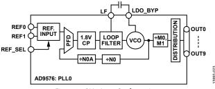
Figure 23. PLL0 Loop Configuration 1
