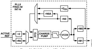
Figure 21. PLL0 Functional Block Diagram
