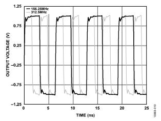
Figure 10. OUT0 Output Waveform, HSTL (156.25 MHz, 312.5 MHz)
