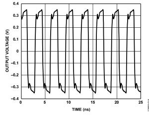
Figure 14. OUT0 Output Waveform, LVDS (312.5 MHz)
