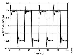
Figure 13. OUT8 Output Waveform, LVDS (133.3 MHz)
