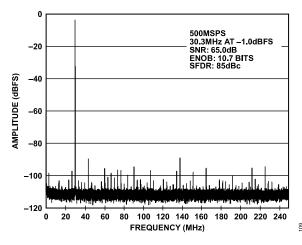
Figure 9. AD9434-500 64k Point Single-Tone FFT; 500 MSPS, 30.3 MHz
