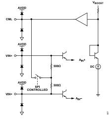
Figure 34. Analog Input DC Equivalent Circuit (V<sub>CML</sub> = ~1.7 V)
