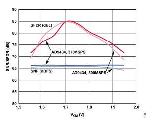
Figure 30. SNR/SFDR vs. Common-Mode Voltage; 370 MSPS, 500 MSPS,  $f_{\rm IN}$  = 140.3 MHz
