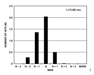
Figure 24. AD9434-370 Grounded Input Histogram; 370 MSPS
