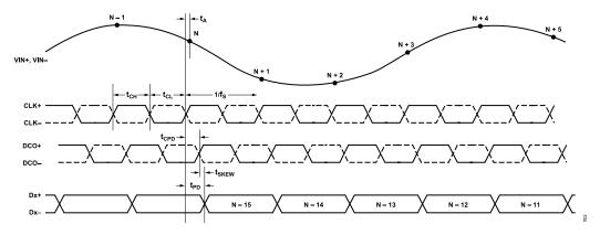
Figure 2. Single Data Rate Mode
