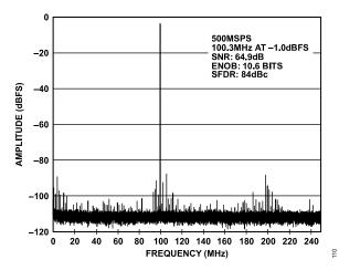
Figure 10. AD9434-500 64k Point Single-Tone FFT; 500 MSPS, 100.3 MHz
