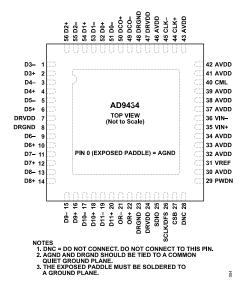
Figure 4. Pin Configuration—Single Data Rate Mode
