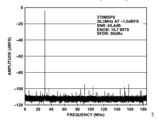
Figure 6. AD9434-370 64k Point Single-Tone FFT; 370 MSPS, 30.3 MHz
