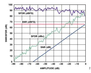
Figure 19. AD9434-500 SNR/SFDR vs. Input Amplitude; 500 MSPS, 140.3 MHz
