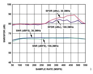
Figure 17. AD9434-500 SNR/SFDR vs. Sample Rate; 30.3 MHz, 100.3 MHz
