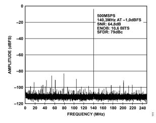
Figure 11. AD9434-500 64k Point Single-Tone FFT; 500 MSPS, 140.3 MHz
