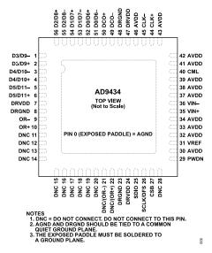
Figure 5. Pin Configuration—Double Data Rate Mode
