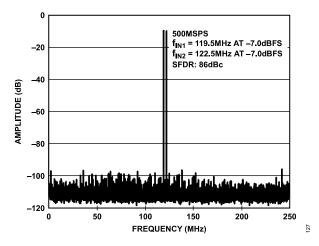
Figure 27. AD9434-500 64k Point, Two-Tone FFT; 500 MSPS, 119.2 MHz, 122.5 MHz
