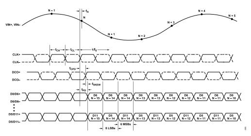
Figure 3. Double Data Rate Mode
