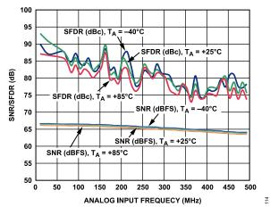
Figure 14. AD9434-370 Single-Tone SNR/SFDR vs. Input Frequency (f<sub>IN</sub>) and Temperature: 370 MSPS
