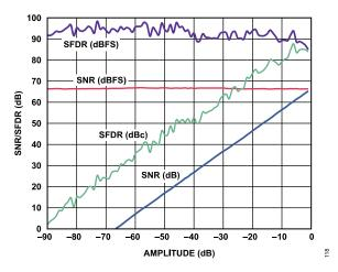
Figure 18. AD9434-370 SNR/SFDR vs. Input Amplitude; 500 MSPS, 140.3 MHz
