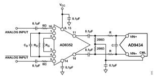
Figure 43. Differential Input Configuration Using the AD8352
