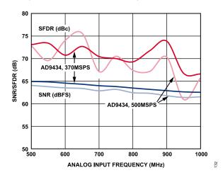
Figure 32. SNR/SFDR for AD9434-370 and AD9434-500 at 370 MSPS and 500 MSPS; AIN Sweep at  $-1.0~\mathrm{dBFS}$
