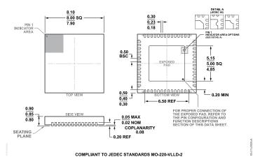
Figure 53. 56-Lead Lead Frame Chip Scale Package [LFCSP] 8 mm × 8 mm Body and 0.85 mm Package Height (CP-56-21) Dimensions shown in millimeters
