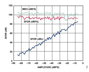
Figure 29. AD9434-500 Two-Tone SFDR vs. Input Amplitude; 500 MSPS, 119.5 MHz, 122.5 MHz
