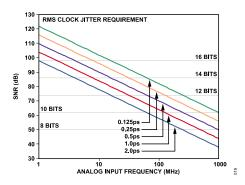
Figure 48. Ideal SNR vs. Input Frequency and Jitter
