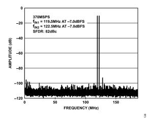
Figure 26. AD9434-370 64k Point, Two-Tone FFT; 370 MSPS, 119.5 MHz, 122.5
