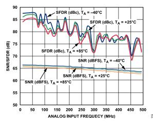
Figure 15. AD9434-500 Single-Tone SNR/SFDR vs. Input Frequency (f<sub>IN</sub>) and Temperature; 500 MSPS
