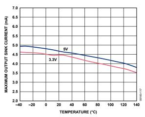
Figure 19. Maximum Output Sink Current vs. Temperature
