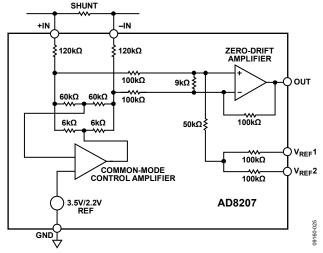
Figure 25. Simplified Schematic
