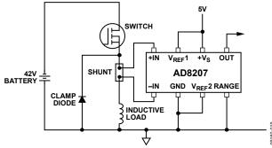
Figure 36. High-Side Switch
