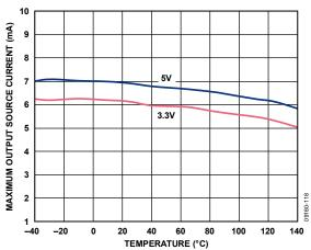
Figure 20. Maximum Output Source Current vs. Temperature
