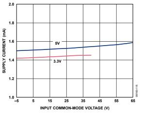
Figure 9. Supply Current vs. Input Common-Mode Voltage
