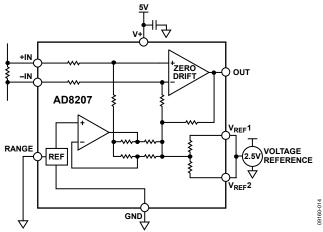
Figure 30. External Referenced Output, V+=5 V
