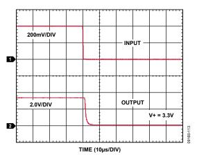
Figure 16. Differential Overload Recovery, Falling (V + = 3.3 V)
