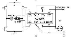
Figure 33. H-Bridge Motor Control Application
