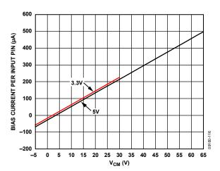
Figure 8. Input Bias Current vs. Common-Mode Voltage
