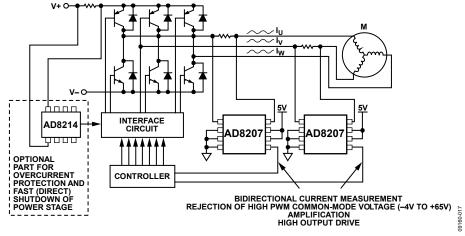
Figure 34. 3-Phase Motor Control
