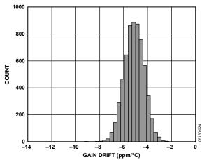
Figure 24. Gain Drift Distribution
