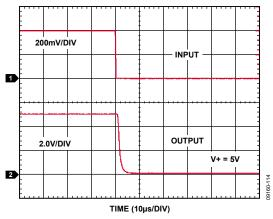
Figure 17. Differential Overload Recovery, Falling (V+=5 V)
