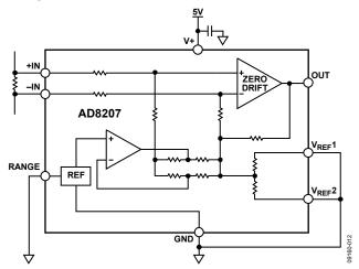
Figure 28. Ground Referenced Output Mode, V+=5 V
