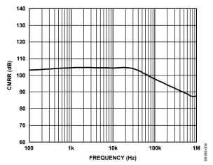
Figure 4. Typical CMRR vs. Frequency
