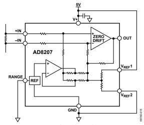
Figure 31. Splitting the Supply, V+=5V
