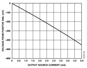
Figure 21. Output Voltage Range vs. Output Source Current
