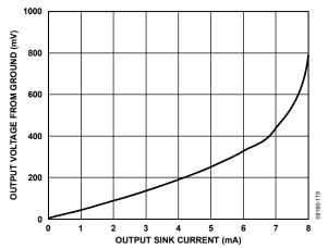
Figure 22. Output Voltage Range from GND vs. Output Sink Current
