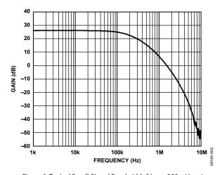
Figure 6. Typical Small-Signal Bandwidth ( $V_{OUT} = 200 \text{ mV } p\text{-}p$ )
