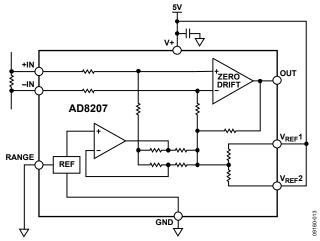
Figure 29. V+ Referenced Output Mode, V+=5V
