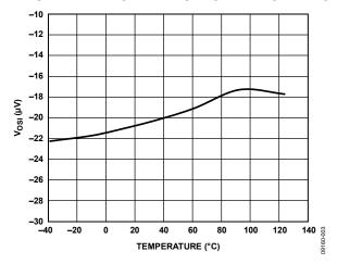
Figure 3. Typical Offset Drift vs. Temperature
