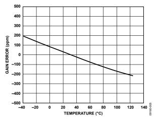
Figure 5. Typical Gain Error vs. Temperature
