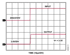
Figure 14. Differential Overload Recovery, Rising (V + = 3.3 V)
