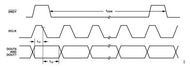
Figure 4. Daisy-Chain Setup and Hold Timing Diagram
