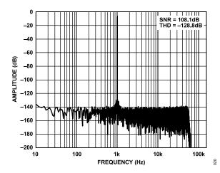
Figure 16. FFT, Median Mode, Wideband Filter, -6 dBFS
