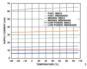
Figure 67. Supply Current vs. Temperature, IOVDD
