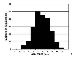
Figure 52. Channel to Channel Gain Error Matching
