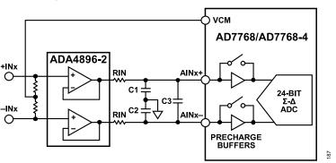
Figure 87. Typical Input Structure for an RC Network
