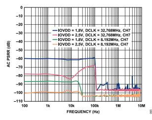
Figure 56. AC PSRR vs. Frequency, IOVDD
