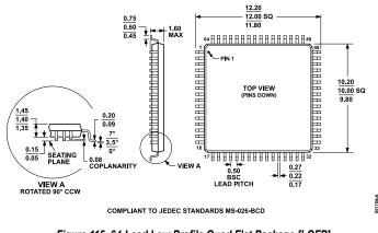
Figure 115. 64-Lead Low Profile Quad Flat Package [LQFP] (ST-64-2) Dimensions shown in millimeters
