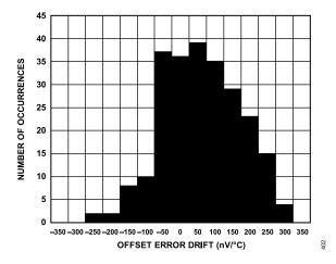
Figure 48. Offset Error Drift, DCLK = 32 MHz
