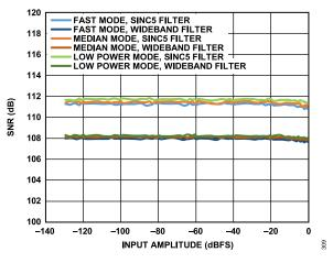
Figure 39. SNR vs. Input Amplitude
