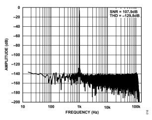
Figure 15. FFT, Fast Mode, Wideband Filter, -6 dBFS
