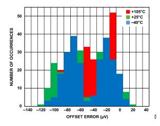
Figure 46. Offset Error Distribution, DCLK = 32 MHz
