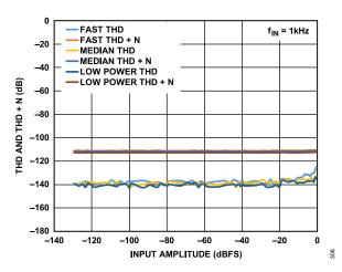
Figure 38. THD and THD + N vs. Input Amplitude, Sinc5 Filter
