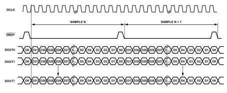
Figure 100. AD7768 FORMATx = 00: Each ADC Has a Dedicated Data Output Pin, Maximum Data Rate
