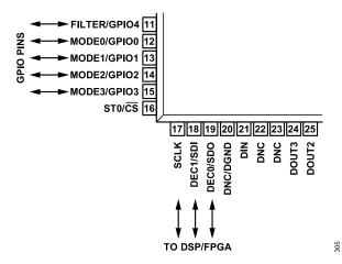
Figure 114. AD7768-4 GPIO Functionality
