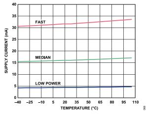
Figure 65. Supply Current vs. Temperature, AVDD1
