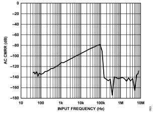
Figure 53. AC CMRR vs. Input Frequency
