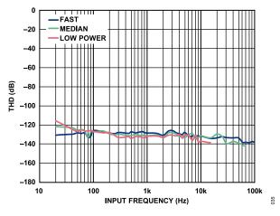
Figure 36. THD vs. Input Frequency, Three Power Modes, Sinc5 Filter
