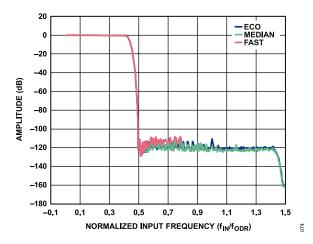
Figure 57. Amplitude vs. Normalized Input Frequency ( $f_{\rm IN}/f_{\rm ODR}$ ), Wideband Filter Profile
