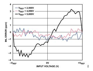
Figure 40. INL Error vs. Input Voltage for Various V<sub>REF</sub> Levels, Fast Mode
