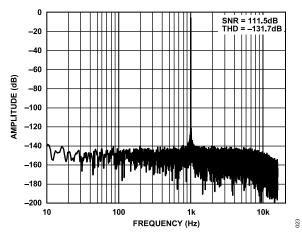
Figure 23. FFT, Low Power Mode, Sinc5 Filter, -6 dBFS
