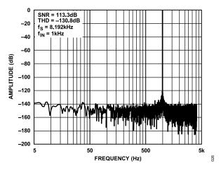
Figure 24. FFT One Shot Mode, Sinc5 Filter, Median Mode, Decimation = ×64, -0.5 dBFS, SYNC IN Frequency = MCLK/4000
