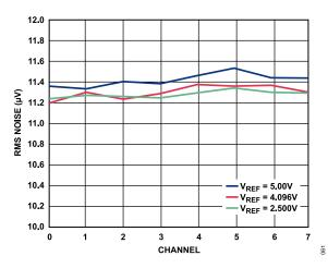
Figure 32. RMS Noise per Channel for Various V<sub>REF</sub> Values
