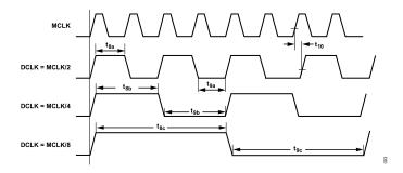
Figure 3. MCLK to DCLK Divider Timing Diagram
