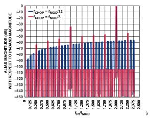
Figure 93. AD7768/AD7768-4 Rejection of Out of Band Input Tones, Wideband Filter, Decimation = ×32, f<sub>MOD</sub> = 8.192 MHz, Analog Input Sweep from DC to 20 MHz
