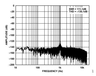
Figure 20. FFT, Low Power Mode, Sinc5 Filter, -0.5 dBFS
