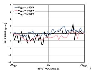
Figure 42. INL Error vs. Input Voltage for Various V<sub>REF</sub> Levels, Low Power Mode
