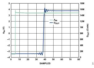
Figure 58. Step Response, Wideband Filter
