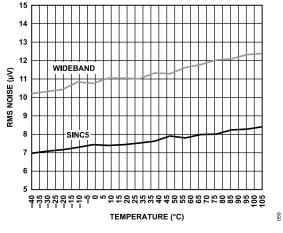
Figure 30. RMS Noise vs. Temperature, Median Mode
