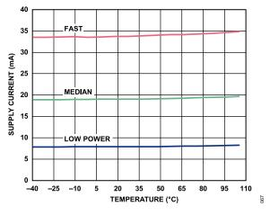
Figure 66. Supply Current vs. Temperature, AVDD2
