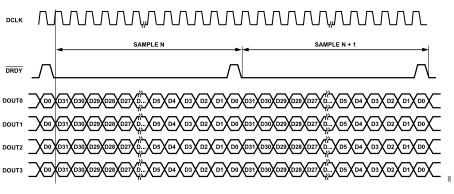
Figure 104. AD7768-4 FORMAT0 = 0: Each ADC Has a Dedicated Data Output Pin, Maximum Data Rate
