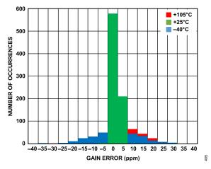
Figure 51. Gain Error Distribution
