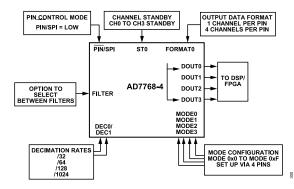
Figure 77. AD7768-4 Pin Configurable Functions
