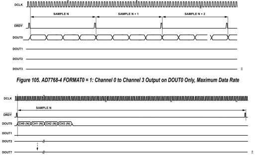
Figure 106. AD7768-4 FORMAT0 = 1: Channel 0 to Channel 3 Output on DOUT0 Only, Decimation = 512
