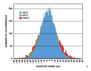
Figure 28. Shorted Noise at Different Temperatures, Wideband Filter
