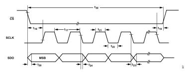
Figure 7. SPI Serial Read Timing Diagram
