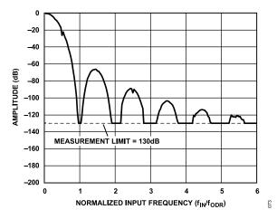
Figure 60. Amplitude vs. Normalized Input Frequency (f<sub>IN</sub>/f<sub>ODR</sub>), Sinc5 Filter Profile
