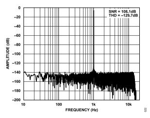
Figure 17. FFT, Low Power Mode, Wideband Filter, -6 dBFS
