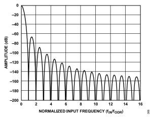
Figure 89. Sinc5 Filter Frequency Response (Decimation = ×32)
