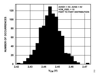
Figure 64. VCM Output Voltage Distribution
