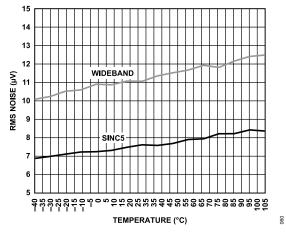
Figure 31. RMS Noise vs. Temperature, Low Power Mode
