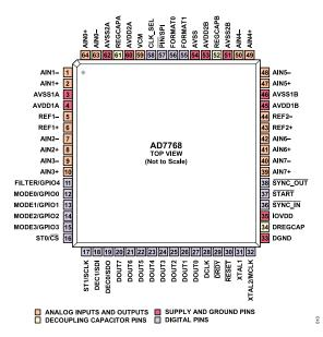
Figure 10. AD7768 Pin Configuration
