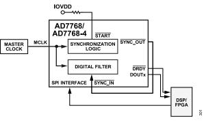
Figure 81. Connection Diagram for Synchronization Using SPI\_SYNC
