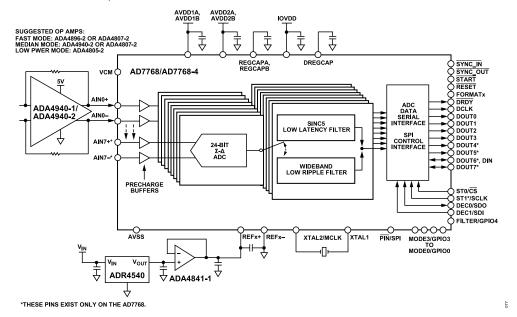
Figure 73. Typical Connection Diagram
