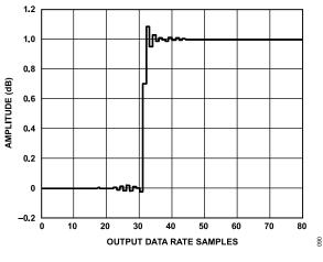
Figure 92. Wideband Filter Step Response
