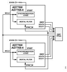
Figure 111. Synchronizing Multiple AD7768/AD7768-4 Devices Using Only SYNC\_IN
