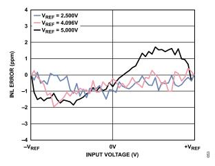
Figure 41. INL Error vs. Input Voltage for Various V<sub>REF</sub> Levels, Median Mode
