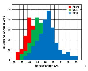
Figure 45. Offset Error Distribution, DCLK = 24 MHz
