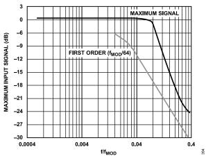
Figure 94. Maximum Input Signal vs. Frequency
