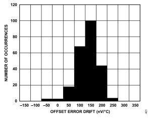
Figure 47. Offset Error Drift, DCLK = 24 MHz
