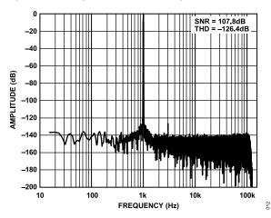
Figure 12. Fast Fourier Transform (FFT), Fast Mode, Wideband Filter, -0.5 dBFS
