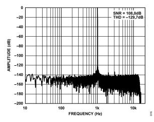
Figure 14. FFT, Low Power Mode, Wideband Filter, -0.5 dBFS
