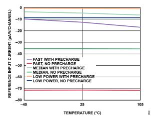
Figure 63. Reference Input Current vs. Temperature, Reference Precharge Buffers On/Off
