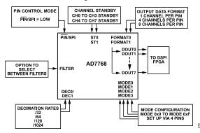
Figure 76. AD7768 Pin Configurable Functions
