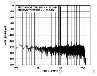
Figure 25. Intermodulation Distortion (IMD) with Input Signals at 9.7 kHz and 10.3 kHz
