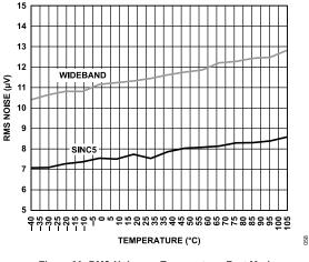
Figure 29. RMS Noise vs. Temperature, Fast Mode
