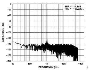
Figure 22. FFT, Median Mode, Sinc5 Filter, -6 dBFS
