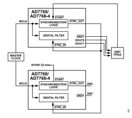
Figure 110. Synchronizing Multiple AD7768/AD7768-4 Devices Using SYNC\_OUT
