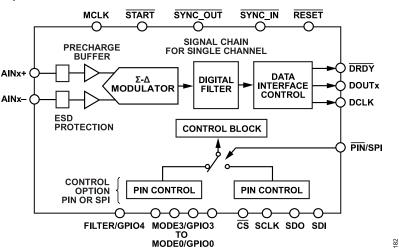
Figure 83. Top Level Core Signal Chain and Control
