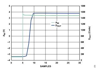
Figure 61. Step Response, Sinc5 Filter
