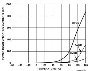
Figure 16. Power-Down Operating Currents vs. Temperature
