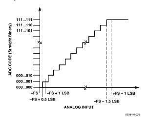
Figure 20. ADC Ideal Transfer Function
