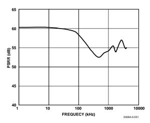
Figure 25. PSRR vs. Frequency
