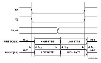
Figure 32. 8-Bit and 16-Bit Parallel Interface
