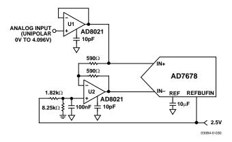
Figure 24. Single-Ended-to-Differential Driver Circuit (Internal Reference Buffer Used)
