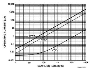
Figure 15. Operating Current vs. Sampling Rate
