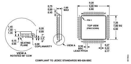
Figure 39. 48-Lead Low Profile Quad Flat Package [LQFP] (ST-48) Dimensions shown in millimeters
