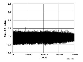
Figure 8. Differential Nonlinearity vs. Code
