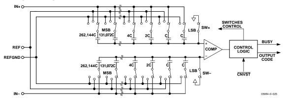
Figure 19. ADC Simplified Schematic
