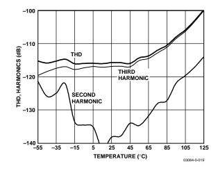
Figure 14. THD and Harmonics vs. Temperature
