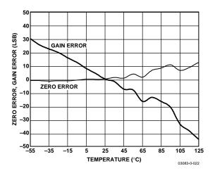
Figure 17. Zero Error and Gain Error vs. Temperature
