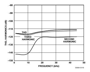
Figure 11. THD and Harmonics vs. Frequency
