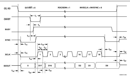
Figure 34. Master Serial Data Timing for Reading (Read Previous Conversion during Convert)
