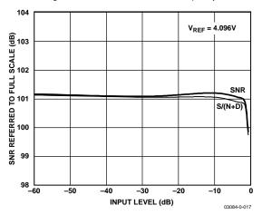
Figure 12. SNR and S/(N+D) vs. Input Level
