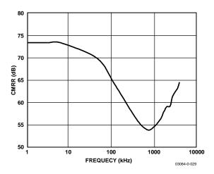
Figure 23. Analog Input CMRR vs. Frequency
