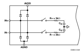
Figure 22. Simplified Analog Input
