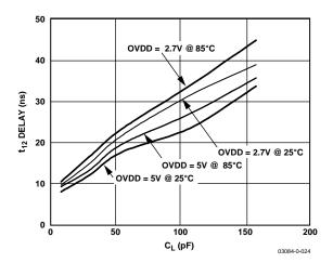
Figure 18. Typical Delay vs. Load Capacitance  $C_L$
