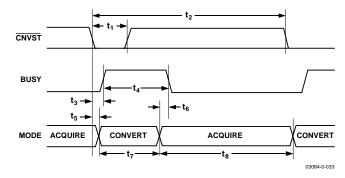
Figure 27. Basic Conversion Timing
