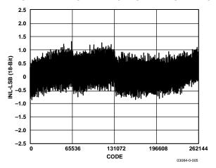
Figure 5. Integral Nonlinearity vs. Code
