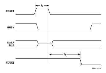
Figure 28. RESET Timing
