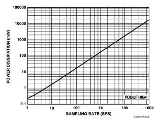
Figure 26. Power Dissipation vs. Sample Rate
