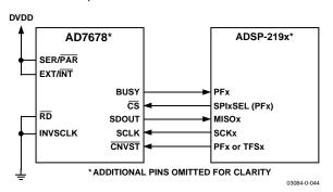
Figure 38. Interfacing the AD7678 to an SPI Interface
