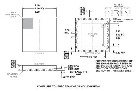
Figure 40. 48-Lead Lead Frame Chip Scale Package [LFCSP] 7 mm × 7 mm Body and 0.75 mm Package Height (CP-48-4) Dimensions shown in millimeters
