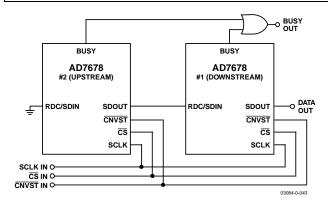
Figure 37. Two AD7678s in a Daisy-Chain Configuration
