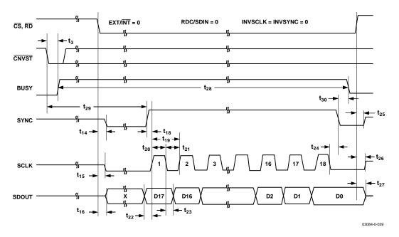
Figure 33. Master Serial Data Timing for Reading (Read after Convert)
