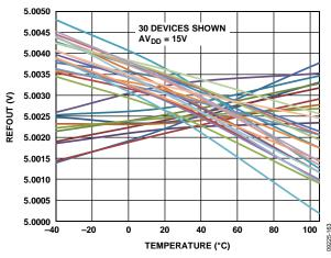
Figure 42. REFOUT vs. Temperature (When the AD5757 is soldered onto a PCB, the reference shifts due to thermal shock on the package. The average output voltage shift is -4 mV. Measurement of these parts after seven days shows that the outputs typically shift back 2 mV toward their initial values. This second shift is due to the relaxation of stress incurred during soldering.)
