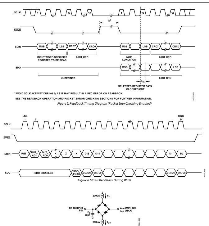
Figure 7. Load Circuit for SDO Timing Diagram
