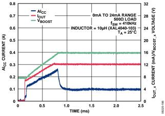
Figure 61. Al<sub>CC</sub> Current vs. Time for 24 mA Step Through 500  $\Omega$  Load with External 51 k $\Omega$  Compensation Resistor
