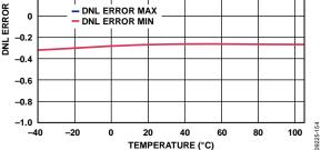
Figure 14. Differential Nonlinearity vs. Temperature
