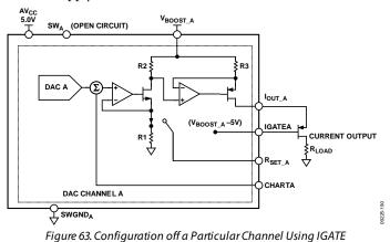
When using the internal  $R_{SET}$  resistor in current output mode, the output is significantly affected by how many other channels using the internal  $R_{SET}$  are enabled and by the dc crosstalk from these channels. The internal  $R_{SET}$  specifications in Table 1 are for all channels enabled with the internal  $R_{SET}$  selected and outputting the same code.
