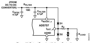
Figure 64. Output Transient Voltage Protection
