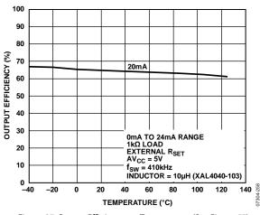
Figure 37. Output Efficiency vs. Temperature (See Figure 57)
