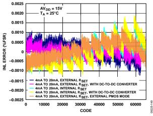
Figure 9. Integral Nonlinearity vs. Code
