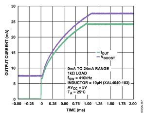
Figure 27. Output Current and V<sub>BOOST\_x</sub> Settling Time with DC-to-DC Converter (See Figure 57)
