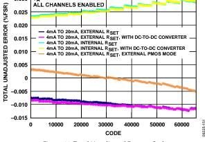
Figure 11. Total Unadjusted Error vs. Code
