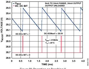
Figure 58. Operation on Reaching V<sub>MAX</sub>
