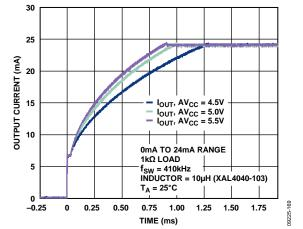
Figure 29. Output Current Settling with DC-to-DC Converter vs. Time and  $AV_{cc}$  (See Figure 57)
