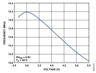
Figure 48. Internal Oscillator Frequency vs. DV<sub>DD</sub> Supply Voltage
