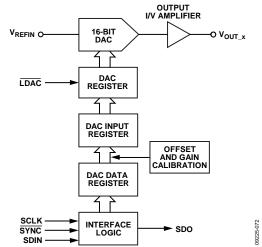
Figure 51. Simplified Serial Interface of Input Loading Circuitry for One DAC Channel
