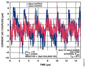
Figure 31. Output Current vs. Time with DC-to-DC Converter (See Figure 57)
