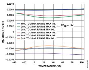
Figure 12. Integral Nonlinearity vs. Temperature, Internal R<sub>SET</sub>
