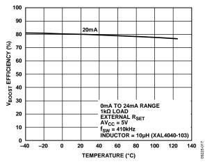
Figure 35. Efficiency at V<sub>BOOST\_x</sub> vs. Temperature (See Figure 57)
