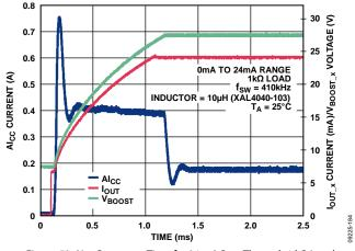
Figure 59. Al<sub>CC</sub> Current vs. Time for 24 mA Step Through 1  $k\Omega$  Load with Internal Compensation Resistor
