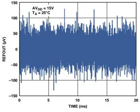
Figure 41. REFOUT Output Noise (100 kHz Bandwidth)
