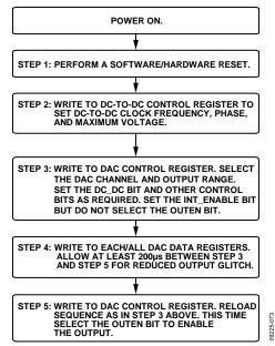
Figure 52. Programming Sequence for Enabling the Output Correctly
