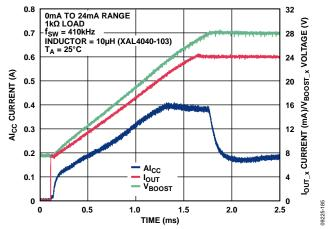
Figure 60. Al<sub>CC</sub> Current vs. Time for 24 mA Step Through 1 k $\Omega$ Load with External 51 k $\Omega$  Compensation Resistor
