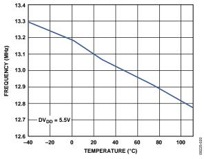
Figure 47. Internal Oscillator Frequency vs. Temperature
