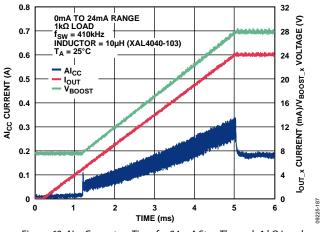
Figure 62. Al<sub>cc</sub> Current vs. Time for 24 mA Step Through 1  $k\Omega$  Load with Slew Rate Control
