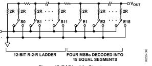
Figure 49. DAC Ladder Structure
