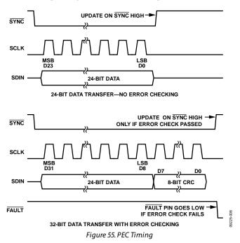
The PEC can be used for both transmit and receive of data packets. If status readback during a write is enabled, ignore the PEC values returned during the status readback during a write operation. If status readback during a write is disabled, the user can still use the normal readback operation to monitor status register activity with PEC.
