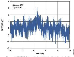
Figure 40. REFOUT Output Noise (0.1 Hz to 10 Hz Bandwidth)
