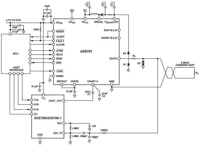
Figure 67. AD5757 in HART Configuration
