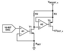
Figure 50. Voltage-to-Current Conversion Circuitry
