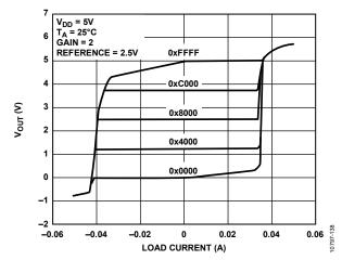
Figure 24. Source and Sink Capability at 5 V
