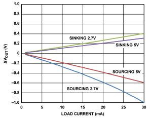
Figure 23. Headroom/Footroom vs. Load Current
