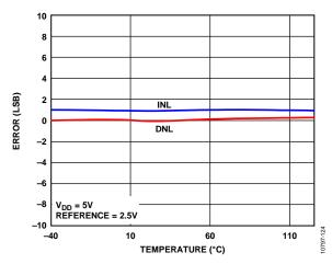
Figure 12. INL Error and DNL Error vs. Temperature
