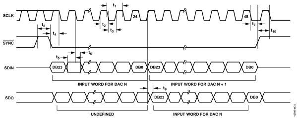
Figure 4. Daisy-Chain Timing Diagram
