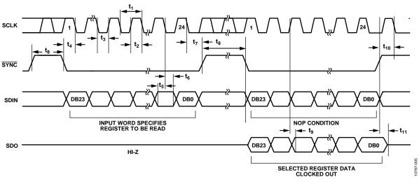
Figure 5. Readback Timing Diagram
