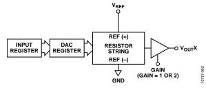
Figure 36. Single DAC Channel Architecture Block Diagram
