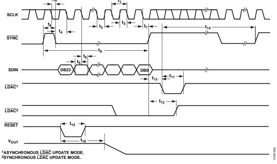
Figure 2. Serial Write Operation
