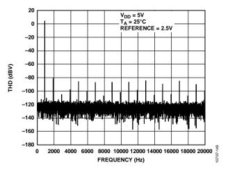
Figure 33. Total Harmonic Distortion @ 1 kHz
