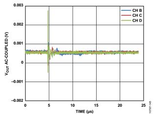
Figure 31. Analog Crosstalk, Channel A
