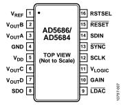
Figure 7. 16-Lead TSSOP Pin Configuration
