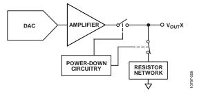
Figure 41. Output Stage During Power-Down
