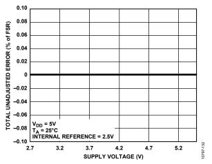
Figure 20. TUE vs. Supply Voltage, Gain = 1
