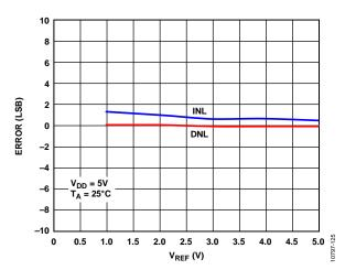
Figure 13. INL Error and DNL Error vs. V<sub>REF</sub>
