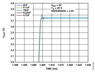
Figure 34. Settling Time vs. Capacitive Load
