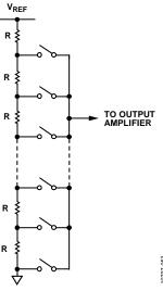
Figure 37. Resistor String Structure
