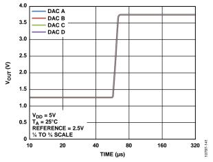
Figure 27. Settling Time, 5 V
