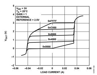
Figure 25. Source and Sink Capability at 3 V
