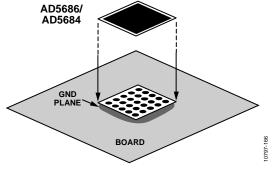
Figure 45. Pad Connection to Board
