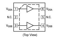
Note: Exposed backside of the package is the source terminal for the transistor.
