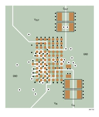
Figure 22. Recommended PCB Layout
