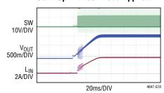
$V_{IN}$  = 12V,  $V_{OUT}$  = 1.2V,  $F_S$  = 500kHz, NO LOAD  $C_{OUT}$  = 1 × 47 $\mu F$  CERAMIC + 1 × 470 $\mu F$  SPCAP  $C_{SS}$  = 0.1 $\mu F$
