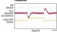
$V_{IN}$  = 12V,  $V_{OUT}$  = 1.8V,  $F_S$  = 700kHz  $C_{OUT}$  = 6 × 100 $\mu$ F CERAMIC 0A to 7.5A LOAD STEP, 10A/ $\mu$ s
