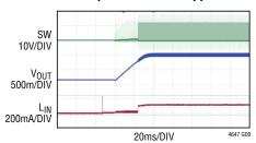
$V_{IN}$  = 12V,  $V_{OUT}$  = 1.2V,  $F_S$  = 500kHz, NO LOAD  $C_{OUT}$  = 1  $\times$  47 $\mu F$  CERAMIC + 1  $\times$  470 $\mu F$  SPCAP  $C_{SS}$  = 0.1 $\mu F$
