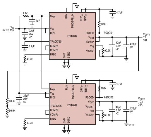
PINS NOT USED IN LTM4647 U1 AND U2 CIRCUITS: CLKOUT, PHASMD, PWM, SW, TEMP<sup>+</sup>, TEMP<sup>-</sup>
