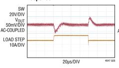
$V_{IN}$  = 12V,  $V_{OUT}$  = 1V,  $F_S$  = 500kHz  $C_{OUT}$  = 6 × 100 $\mu$ F CERAMIC 0A to 7.5A LOAD STEP, 10A/ $\mu$ S
