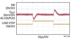
$V_{IN}$  = 12V,  $V_{OUT}$  = 1.2V,  $F_S$  = 500kHz  $C_{OUT}$  = 6 × 100 $\mu$ F CERAMIC 0A to 7.5A LOAD STEP, 10A/ $\mu$ s
