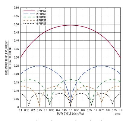
Figure 4. Normalized Input RMS Ripple Current vs Duty Cycle for One to Six µModule Regulators (Phases)
