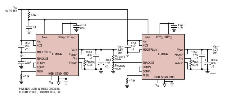
Figure 6. Example Schematic of Ratiometric Output Voltage Tracking
