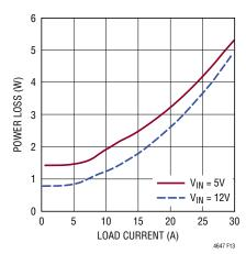
Figure 13. 1.5V Power Loss Curve
