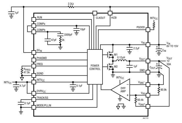
Figure 1. Simplified LTM4647 Block Diagram
