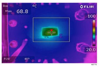
Figure 10. LTM4647 12V  $_{\mbox{\footnotesize{IN}}}$  to 1V  $_{\mbox{\footnotesize{OUT}}}$  at 30A with No Air Flow and No Heat Sink
