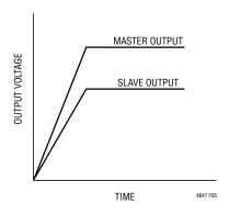
Figure 5. Output Ratiometric Tracking Waveform
