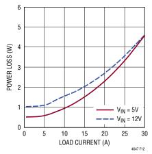
Figure 12. 1.0V Power Loss Curve
