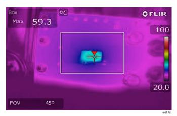
Figure 11. LTM4647 12V  $_{\mbox{\footnotesize IN}}$  to 1V  $_{\mbox{\footnotesize OUT}}$  at 30A with 200LFM Air Flow and No Heat Sink
