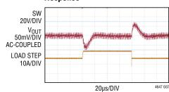
$V_{IN}$  = 12V,  $V_{OUT}$  = 1.5V,  $F_S$  = 600kHz  $C_{OUT}$  = 6 × 100 $\mu F$  CERAMIC 0A to 7.5A LOAD STEP, 10A/ $\mu s$
