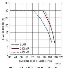
Figure 16. 12V to 1V Derating Curve, BGA Heat Sink
