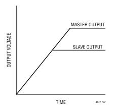
Figure 7. Output Coincident Tracking Waveform
