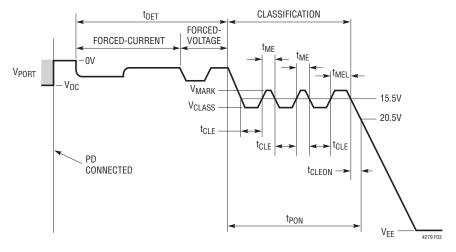
Figure 3. Detect, Three Event Class and Turn-On Timing
