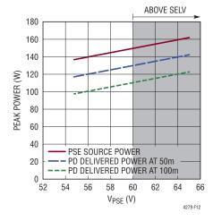
Figure 12. UltraPWR Power vs V<sub>PSE</sub>
