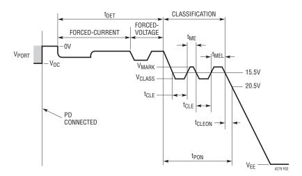
Figure 2. Detect, Two Event Class and Turn-On Timing
