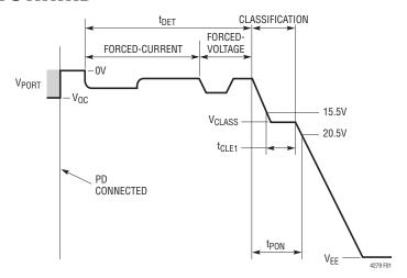
Figure 1. Detect, Single Event Class and Turn-On Timing
