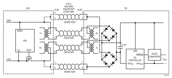
Figure 6. Power over Ethernet System Diagram
